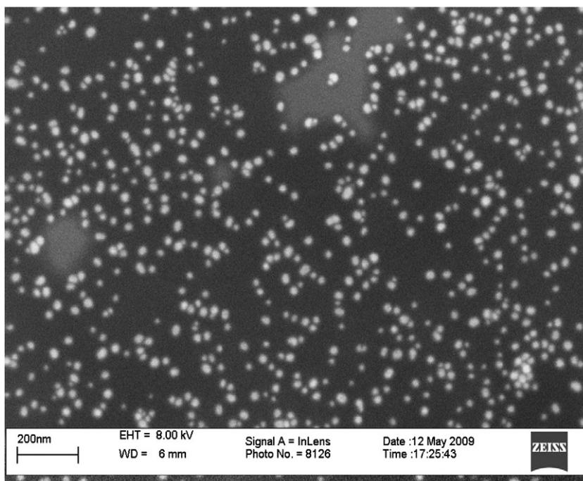
**Fig. 2.** Scanning electron monographs of the prepared AuNPs. One drop of AuNPs was placed on silicon slide and left to dry then examined using field emission scanning electron microscopy (Model: Leo Supra 55).
